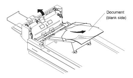
Figure 4.2 ADF Paper Jam - Removing the Paper
